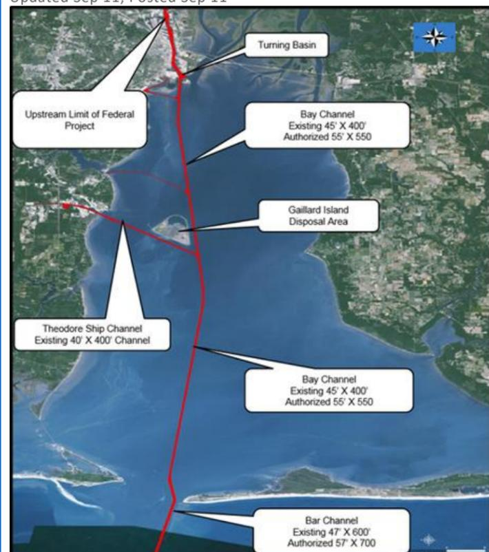
A Corps of Engineers image shows the areas affected by a plan to enlarge the ship channel that connects the Port of Mobile to the Gulf of Mexico. (USACE)
