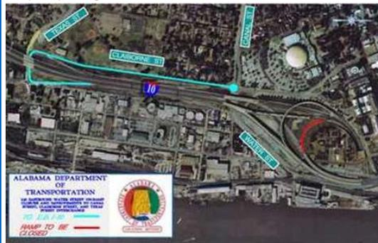
In this ALDOT illustration, the red arc shows the current on-ramp from Water Street to eastbound I-10, which would be closed. The hook-shaped blue line shows the suggested path of tunnel traffic along Claiborne Street to Texas Street, where it would turn back toward downtown and merge onto I-10 using a straight ramp. (Courtesy of ALDOT)
