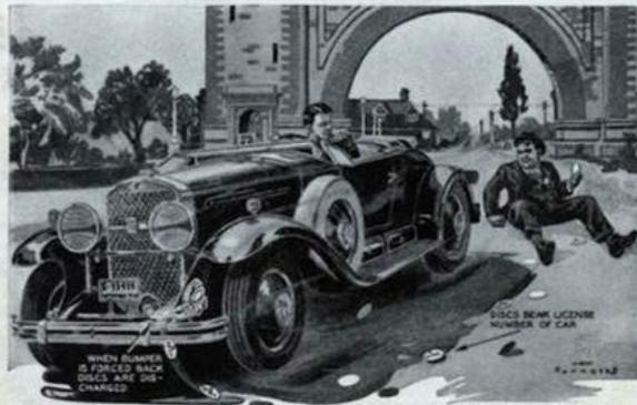
This drawing shows how victim can identify hit and run driver by disks discharged from bumper. Disks get discharged from car when incident occurs...
